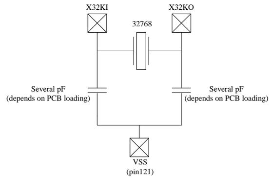
A Crystal (32768Hz) may be used for applications that may involve with precise time clock requirement. See the above diagram for more details.
